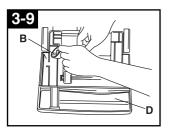
With lettering on outside of belt and positioned as shown in box on (D), slide new belt over motor pulley (B).
